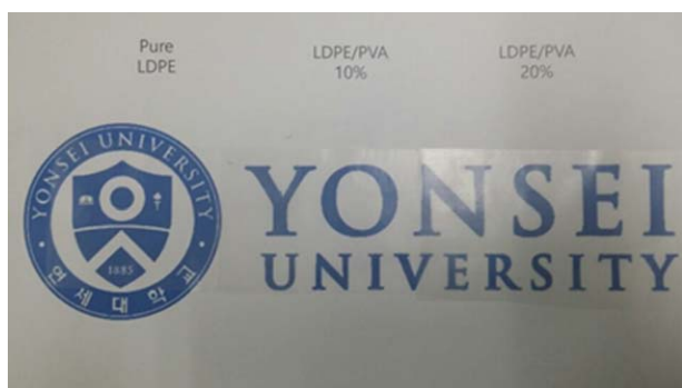
Figure 1. Photograph images of the glycerin-plasticized LDPE/PVA blend films. [Color figure can be viewed in the online issue, which is available at wileyonlinelibrary.com .]
